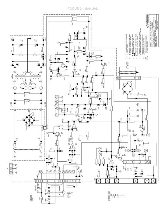
Figure 24: Schematic Diagram Main PC Board, 2450-1000, Rev.C
