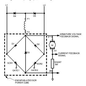
Figure 7: Power Bridge Assembly
