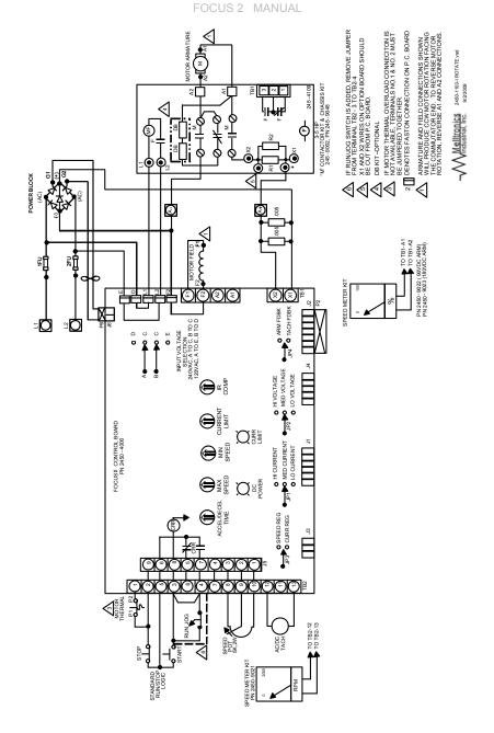
Figure 17: Panel Mount & Less Operators High HP Controls with "M" Contactor,2450-1103-I,Rev.A
