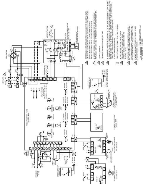
Figure 22: Enclosed Low HP Control with Reversing Kit, 2450-1004-I, Rev. A
