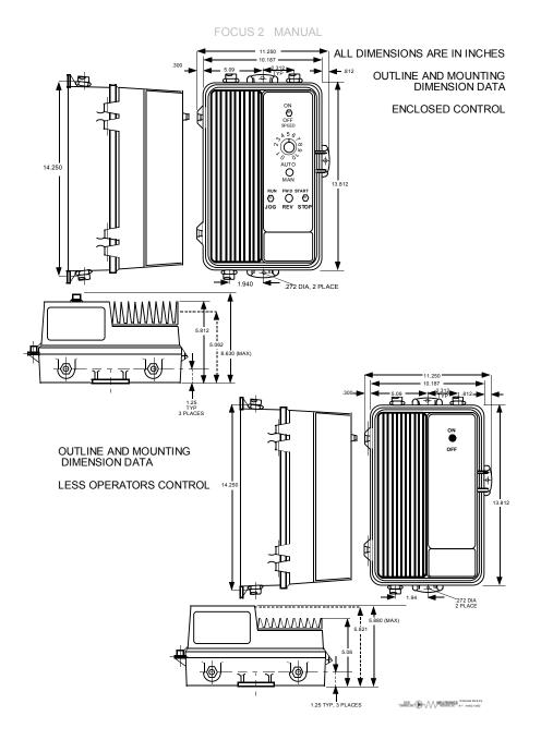
Figure 10: Outline and Mounting Dimensions for Enclosed Controls
