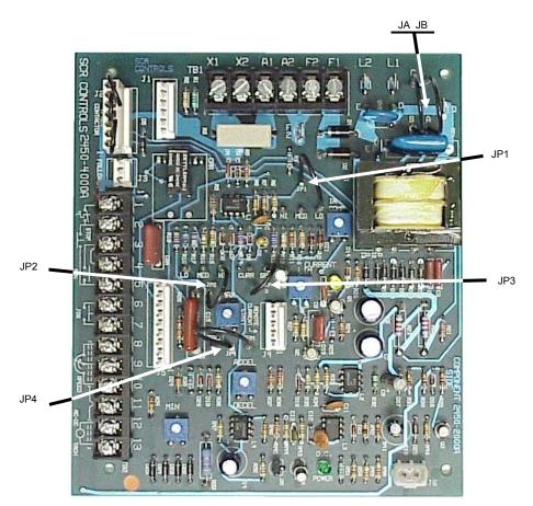
Figure 5: Main PC Board Jumper Locations
