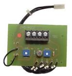
Remote Current Limit/Torque Taper
