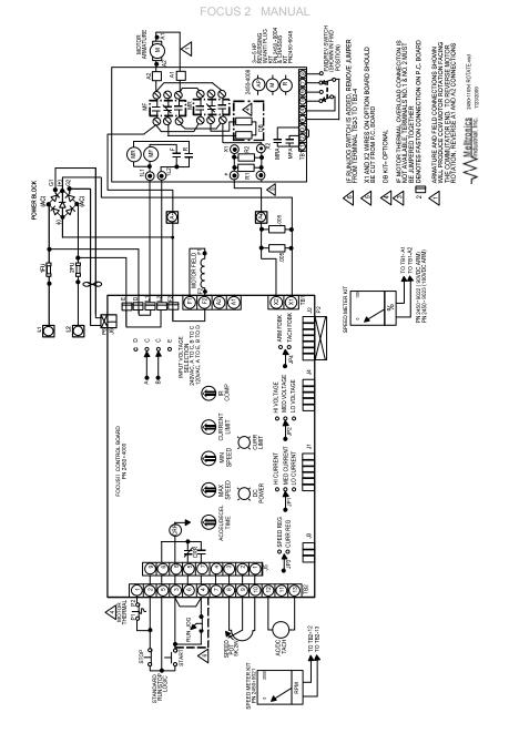
Figure 19: Panel Mount & Less Operators High HP Controls with Reversing Kit,2450-1105-I,Rev.A
